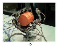
Figure 1. Robotic hand. (a) tendon driven system, bending and pressure sensors. (b) grasping an object.
